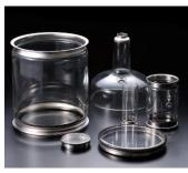
We have a wide lineup of GTMS (glass-to-metal sealing) products. We realize excellent hermeticity by ringsealing or glass frit bonding (Helium leak rate:  $1 \times 10^{-11} \text{ Pa} \cdot \text{m}^3/\text{s}$ or less) and provide these products for highvacuum applications.
