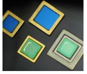
A type of glass LID in which a glass window is joined to a metal frame with sealing glass. Silica glass, sapphire, Si, Ge, etc. can also be joined with appropriate sealing glass.
